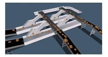
A loop sortation system can be fed manually or automatically from a singulated flow of packages.
